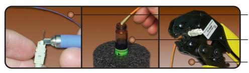
New cleave tool features a double-sided sapphire blade to provide twice the usable life
